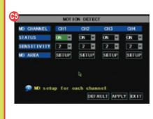
The Motion detection Menu (C5) has three sections, including Channel Status, Sensitivity and Motion area. <u>CHANNEL STATUS:</u> This option allows you to enable motion detection on any channel. <u>SENSITIVITY:</u> This option allows you to set the sensitivity level of motion detection from 1 to 4.
